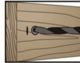
Drill a hole.
